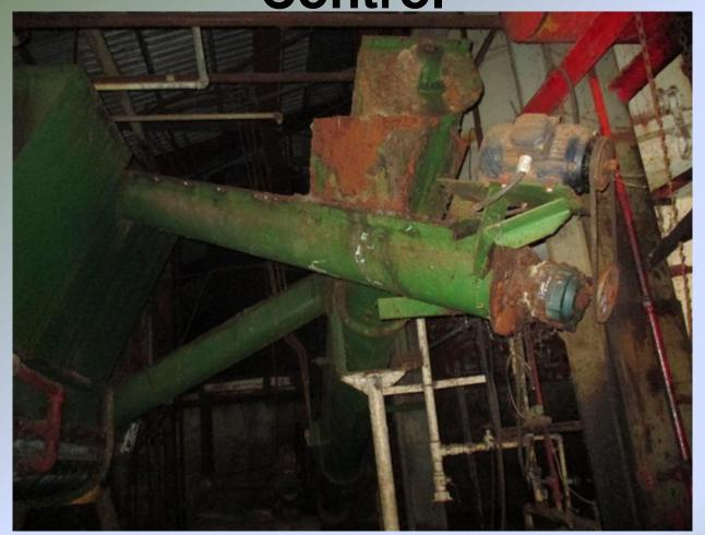
Screw Conveyor 12 in. x 25 ft. with Motor, Gearbox and Electrical Control
