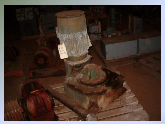
25 hp Lighting tank agitator with blade 15 ft. diameter fiberglass tank tank tapered bottom 25 ft. high
