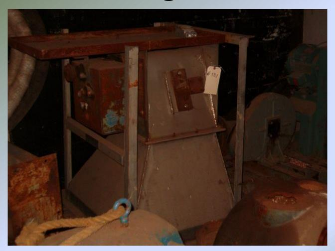
Rietz 40 HP Vertical Grinder with Feed Hopper 8 ft. x 8 ft. 5 ft. Deep and 12 in. Feed Auger and 5 ft. 12 in.
