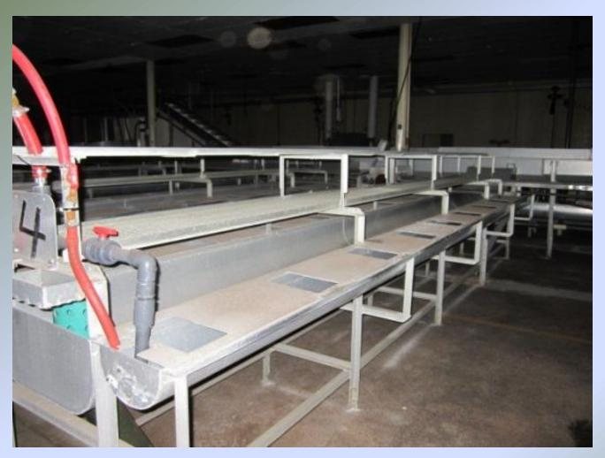
Stainless Steel Dip Pan 2 ft. x 3 ft. 9 in. deep with Frame; Aluminum Table 2 ft. x 4 ft; Stainless Steel Table Top 44 in. x 8 ft.
