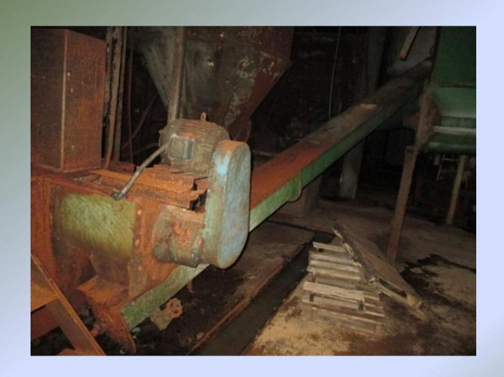
Screw Conveyor 12 in. x 12 ft. with Motor, Gearbox and Electrical Control
