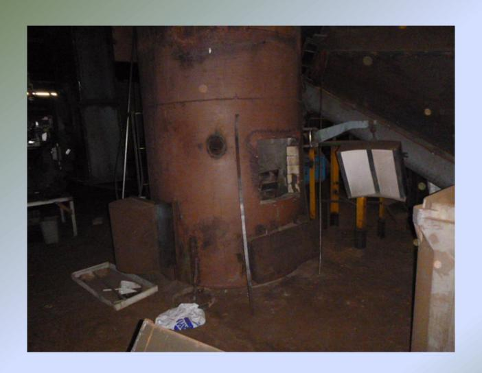
Stord Bartz Stainless Steel Tube Three Stage Falling Film Evaporator 750 MT/Day Capacity with 3 Viking 6 in. 15 HP Circulating Pumps, Vacuum Pump Sihi 25 HP, Gould 2 in. Condensate Pump with 3 HP Motor, Viking 2 in. Stick Water Pump with 3 HP motor, Control Panel, Barometric Condenser, Piping, Structural Steel and Electrical Control
