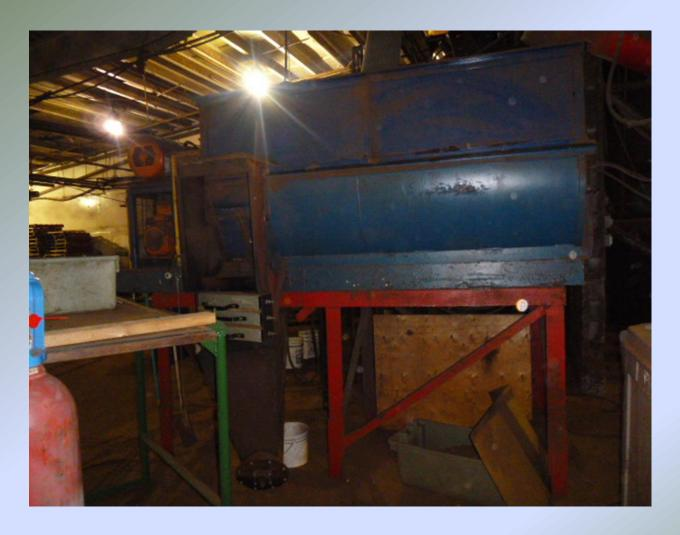
Wire wedge dewatering screen 4 ft. length, 24 in. diameter with motor gearbox
