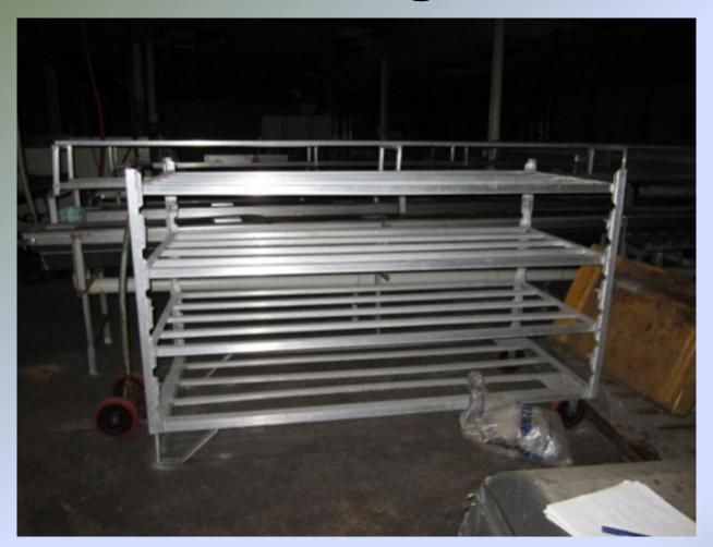
Blast Freezer Rack 3 ft. Wide x 7 ft. Long x 4 ft. High with 5 in. Spacing -
