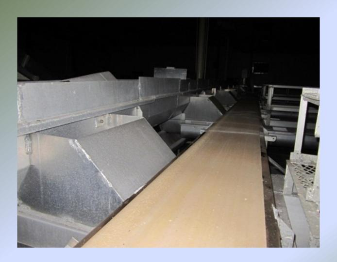
Fishmeal PreserHolding Bin 12 ft. x 12 ft. by 10 ft. High with 12 in. Auger and 10 ft. Long Discharge Screw Conveyor Motors, Gearboxes and Electrical Controls vative Metering Feeder
