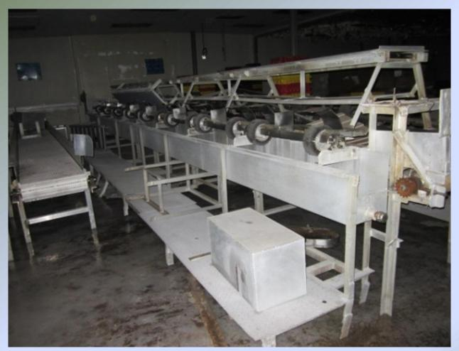
Snow Crab Butchering Conveyor 32 Station 32 ft. Long x 10 ft. Wide with Stands, Motor, Gearbox, Piping and Electrical Control
