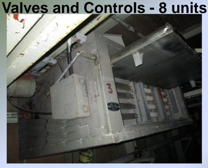
Stainless Steel Chill Cooling Tank (Cools 100,000 lbs of Snow Crab in 10 hrs.) with Moving Conveyor and Motors, Gearboxes,
