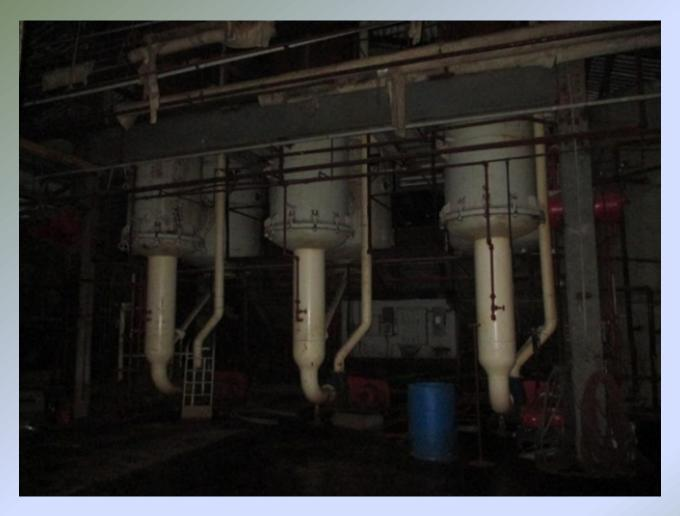
Stord Bartz Stainless Steel Tube Three Stage Falling Film Evaporator 750 MT/Day Capacity with 3 Viking 6 in. 15 HP Circulating Pumps, Vacuum Pump Sihi 25 HP, Gould 2 in. Condensate Pump with 3 HP Motor, Viking 2 in. Stick Water Pump with 3 HP motor, Control Panel, Barometric Condenser, Piping, Structural Steel and Electrical Control
