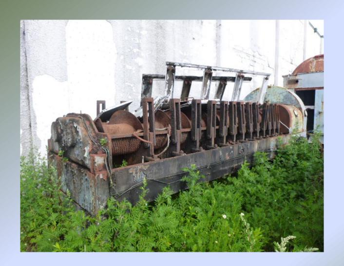
Fish Waste Cooker 300 Mt /Day Capacity 3 ft. Diameter 27 ft. Long with Motor, Gear Box and Electrical Control
